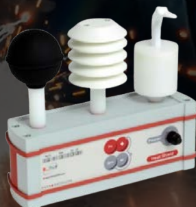
Heat Shield satellite modules Small black globe sphere (5 cm diameter).
