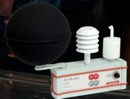
Heat Shield satellite modules Large black globe sphere (15 cm diameter).
