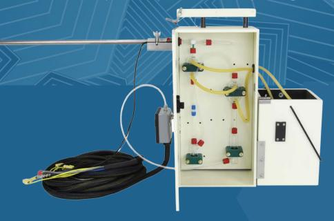
The Apex Instruments SuperVOST Sampling Kit includes the multifunctional VersaCase2 cabinet with a redesigned mounting panel, glass-lined probe assembly, VOST glassware with clamps, insulated coolant reservoir with a submersible pump and VU-cord. The VU-cord can be used for connection directly to the Model 623 Source Sampler Console, or to Model 572 with the VUA orifice flow adapter.
